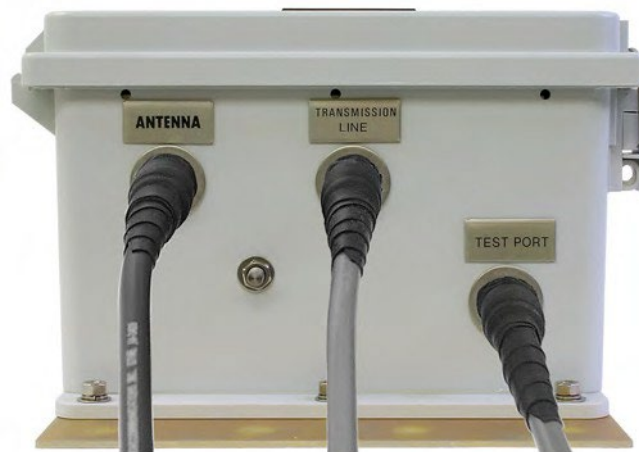
Figure 13: Application of rubber splicing tape. NOTE: Additional waterproofing protection can be realized by covering the rubber tape with either "Scotch Kote" or vinyl plastic electrical tape ("Scotch" brand 33+).
