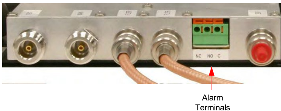
Figure 14: Alarm terminals. Normally open and normally closed terminals are available.
